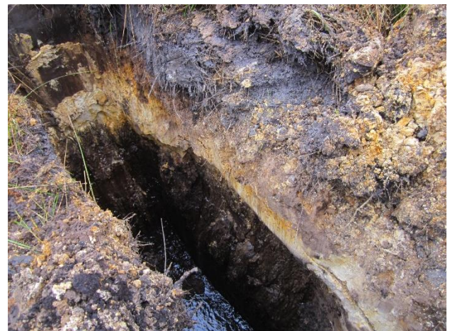
TP6 – Test pit near southern boundary. Perched water table inflow occurring in peat horizon above shallow indurated sand horizon. Water inflow also occurring above deeper indurated sand horizon.
